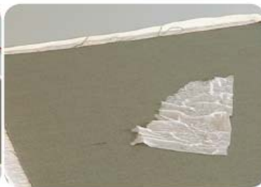
After 28 seconds the textile surface is dry, and most of the water has been removed from the paper on top.
