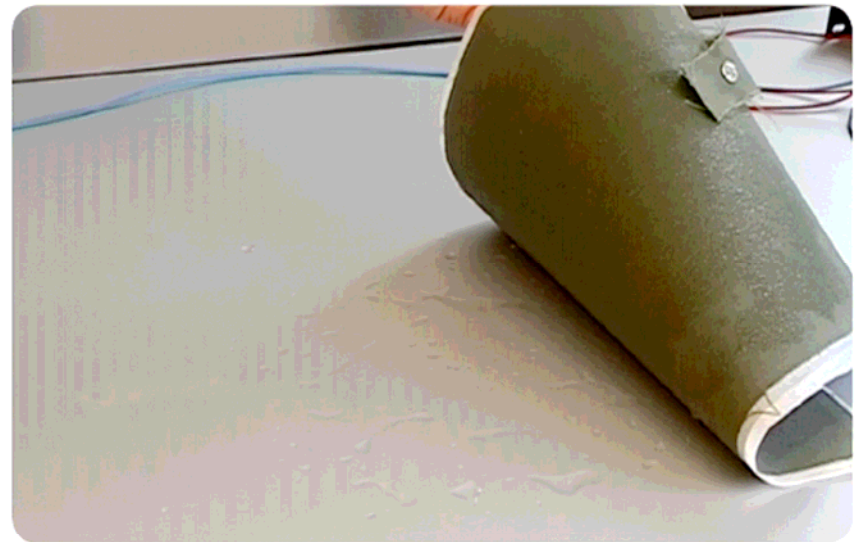
The water has been transported through the textile. In applications the water will run off. In this demonstration, the power consumption was about 5W. When dry, the power consumption falls to zero.
